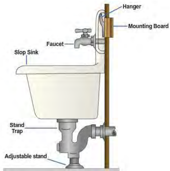
Figure 6-13 – Service (slop) sink.
