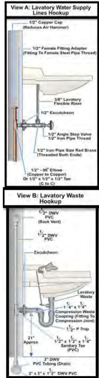
Figure 6-15 – Lavatory water supply and waste hookups.
